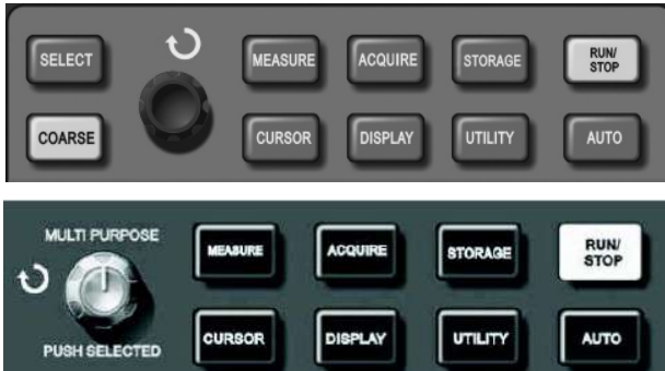
Figure 2–27 Function key (and function) of sampling
