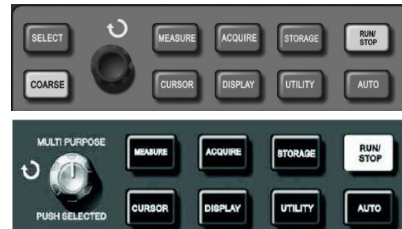
Figure 2-29 Function key (or cursor) of sampling system
