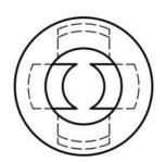
MOUNTING HOLE Ø4.5 CHASSIS THICKNESS 0.8~1.2
