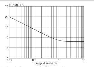
Fig.5. Maximum permissible repetitive rms on-state current  $I_{T(RMS)}$ , versus surge duration, for sinusoidal currents, f = 50 Hz;  $T_{mb} \le 102$  °C.
