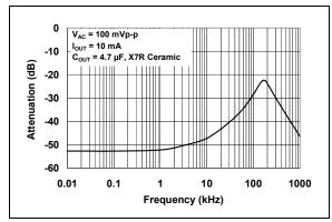
**FIGURE 2-11:** Power Supply Ripple Rejection (PSRR).
