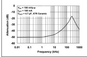
**FIGURE 2-12:** Power Supply Ripple Rejection (PSRR).
