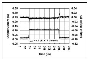
FIGURE 2-15: Load Transient Response.
