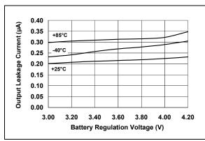
**FIGURE 2-3:** Output Leakage Current  $(I_{DISCHARGE})$  vs. Battery Regulation Voltage  $(V_{BAT})$ .
