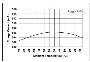
**FIGURE 2-8:** Charge Current ( $I_{OUT}$ ) vs. Ambient Temperature ( $T_A$ ).
