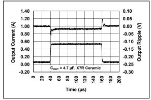
FIGURE 2-16: Load Transient Response.
