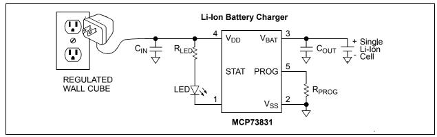
FIGURE 6-1: Typical Application Circuit.
