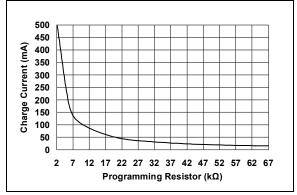
**FIGURE 2-4:** Charge Current  $(I_{OUT})$  vs. Programming Resistor  $(R_{PROG})$ .
