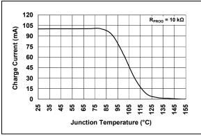
**FIGURE 2-9:** Charge Current  $(I_{OUT})$  vs. Junction Temperature  $(T_1)$ .
