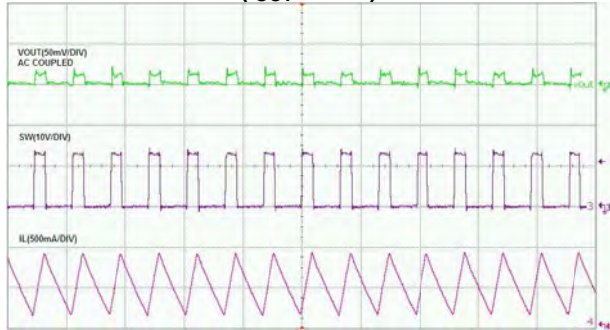
Steady State Test ( I_{OUT} = 0.5A )
