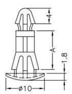
HOLE IN CHASSIS Ø5.5 CHASSIS THICKNESS 1.2~1.8
